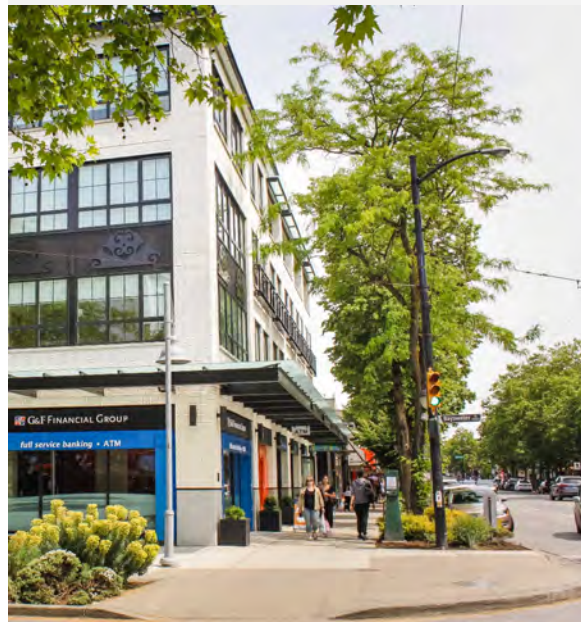
A block that successfully meets several criteria, including zero setback, shading street trees, on-street parking, active ground floor uses, and weather protection above entrances. Note that overhead weather protection can take many forms, including cloth awnings and fixed canopies such as shown above.
