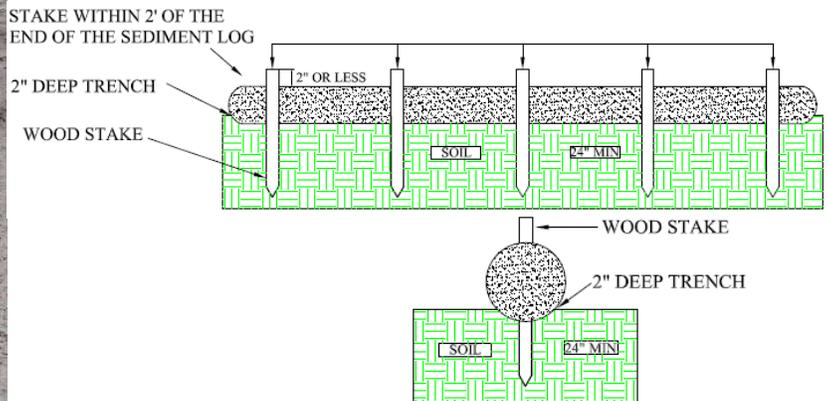
**Sediment logs (also called bio-rolls or wattles)** are made of straw or wood fiber bound within a net to form a tube.
