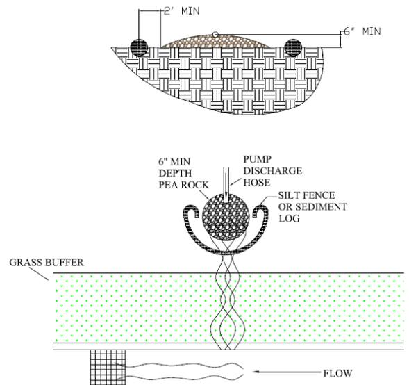
The solution for instances where construction site water must be pumped is to use filter bags, socks or temporary sediment basin.
