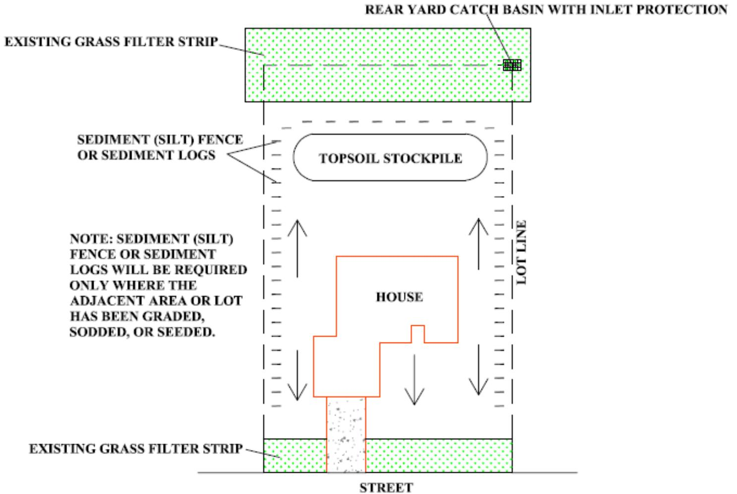
**NOTE: SEDIMENT (SILT) FENCE OR SEDIMENT LOGS WILL BE REQUIRED ONLY WHERE THE ADJACENT AREA OR LOT HAS BEEN GRADED, SODDED, OR SEEDED.**
