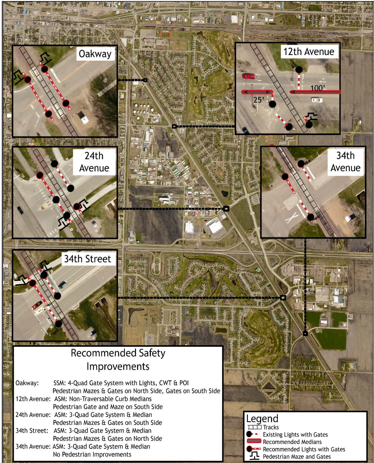
Figure 3 - Recommended Risk Reduction Method for Proposed OTVR Quiet Zone
