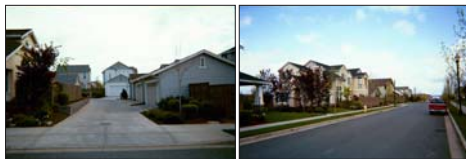
Houses on two streets share driveways in Hillsboro, Oregon. The shared driveways reduce the number of driveways to only one or two per block.
